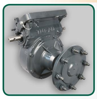
The UMC® TNT-UV-AD™ gearbox is purpose built for higher performance and longer life. It features a 52:1 gear ratio, a 2.25" diameter output shaft, large input bearings, cartridge seals and enhanced gear material that allows for increased load capacity, reduced gear wear and lower operating temperatures. It is a direct replacement for its predecessor, the TNT-2-UV™.
