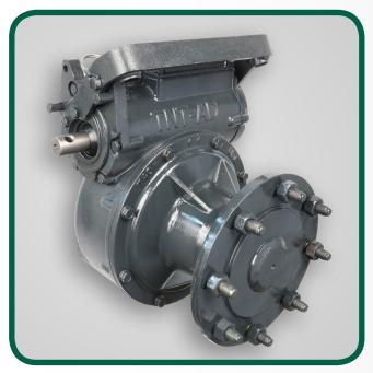
The UMC® TNT-U-AD<sup>™</sup> gearbox is purpose built for higher performance and longer life. It features a 50:1 gear ratio, a 2.25" diameter output shaft, large input bearings, cartridge seals and enhanced gear material that allows for increased load capacity, reduced gear wear and lower operating temperatures. It is a direct replacement for its predecessor, the TNT-2-U<sup>™</sup>.
