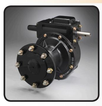
The UMC® 740-UV™ gearbox features a 52:1 gear ratio, a 2.25" diameter extended output shaft, large input bearings, cartridge seals and enhanced gear material that allows for increased load capacity, reduced gear wear and lower operating temperatures.
