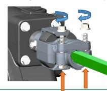
The illustration shown is using a 0.75 inch square shaft (configuration 1) as an example.
