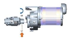
3. Before installing the drive shaft, align the CX Couplers axially by rotating the already installed coupler on the center drive's side. Once aligned, install the square shaft onto the two couplers in one of the two shaft configurations shown. Center the shaft for even gaps on both ends.
