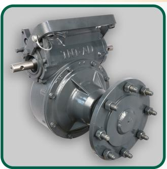
The UMC® TNT-UV-AD<sup>™</sup> gearbox is purpose built for higher performance and longer life. It features a 52:1 gear ratio, a 2.25 inch diameter output shaft, large input bearings, cartridge seals and enhanced gear material that allows for increased load capacity, reduced gear wear and lower operating temperatures. It is a direct replacement for its predecessor, the TNT-2-UV<sup>™</sup>.
