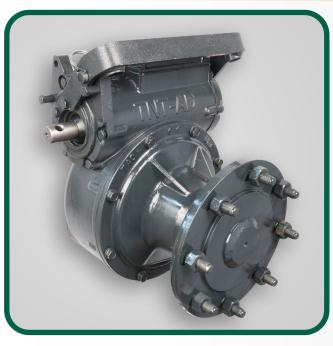
The UMC® TNT-U-AD™ gearbox is designed for use on towable center pivots and lateral/linear irrigation systems. The gearbox design allows the worm gear to disengage from the bull gear so the output shaft can rotate freely, enabling users to move irrigation systems from one field to another.
