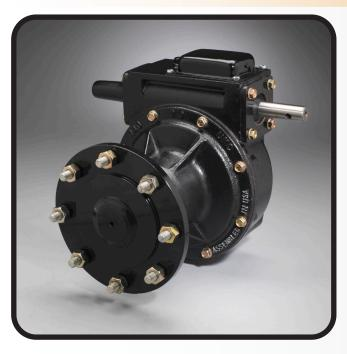
The UMC® 740-UV™ gearbox features a 52:1 gear ratio, a 2.25 inch diameter extended output shaft, large input bearings, cartridge seals and enhanced gear material that allows for increased load capacity, reduced gear wear and lower operating temperatures.
