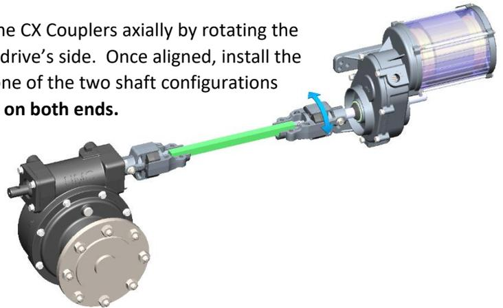
4. Once the drive shaft is in place, re-install the saddle mount and insert the two bolts. Tighten the two nuts in an **ALTERNATING FASHION, one full turn at a time to avoid damaging the Saddle Mount.** Tighten to 35 ft-lbs. of torque. **DO NOT OVER-TIGHTEN.**
