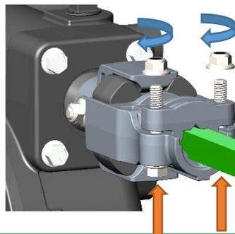
*The illustration shown is using a 0.75 inch square shaft (configuration 1) as an example.*
